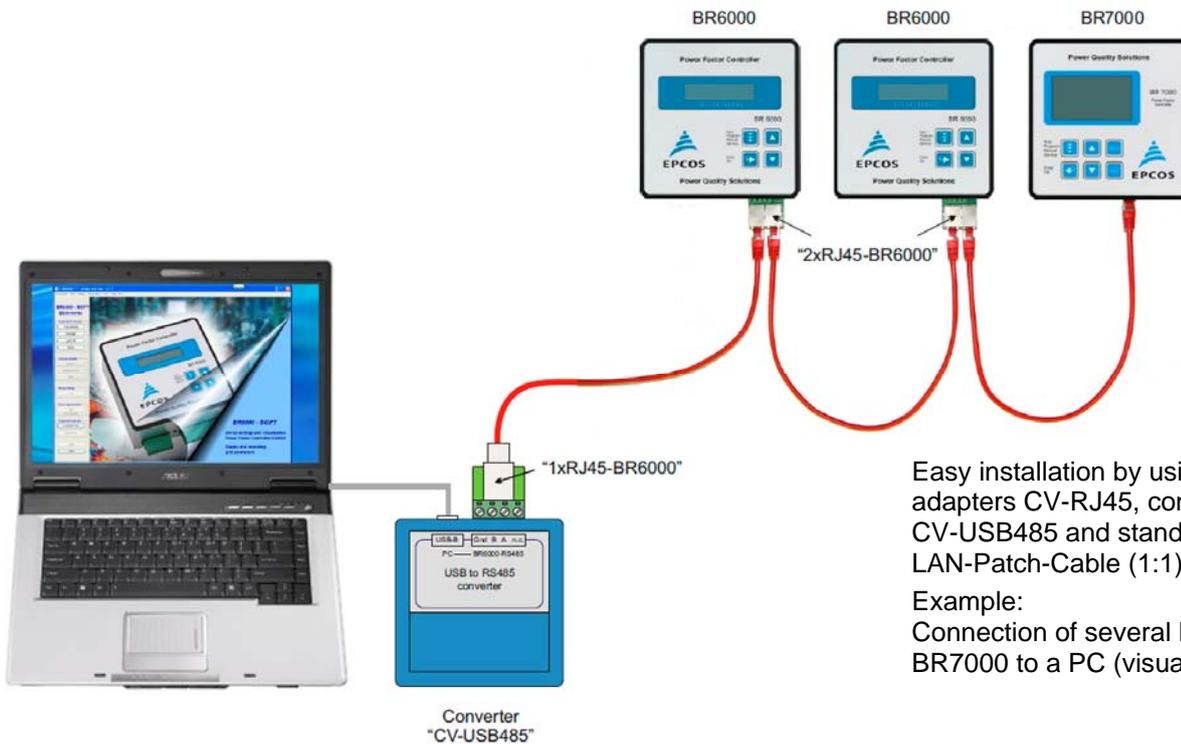
Easy installation by using adapters CV-RJ45, converter CV-USB485 and standard LAN-Patch-Cable (1:1)
